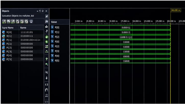
Figure 9: Simulation Waveform of Proposed Multiplier Showing Input and Output Signals
