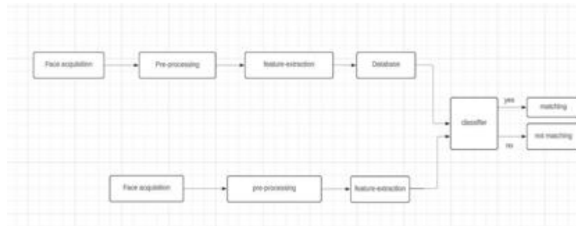
Figure 1: Proposed block diagram
