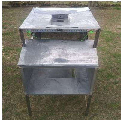
Figure 2: The machine's frame, constructed from mild steel, provides stability and support for all key components
