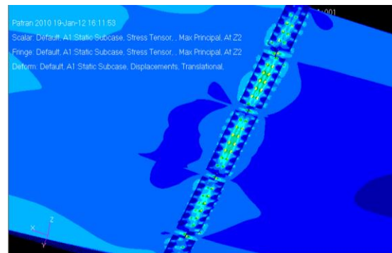
Figure 3(b): maximum stress concentration at bottom skin splice joint
