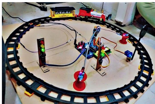
Figure: Railway gate crossing and crack detection
