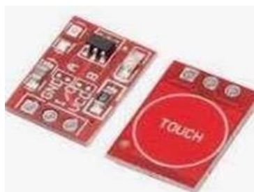
Figure7: Touch sensor used as a switch
