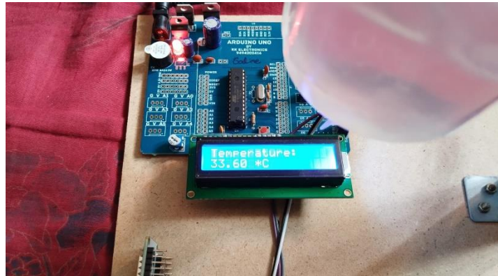
Figure 10: Output on the LCD indicating temperature of the patient
