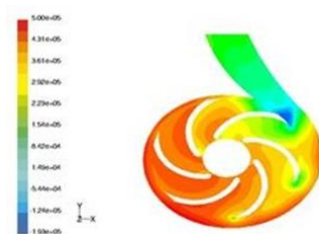
Figure 1: CFD Result for existing single volute centrifugal pump
