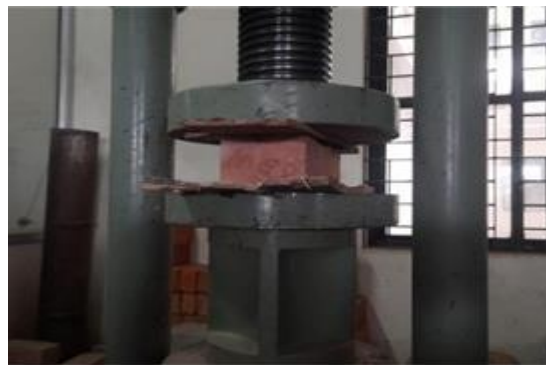
Figure 3: Compressive Strength Testing On Brick
