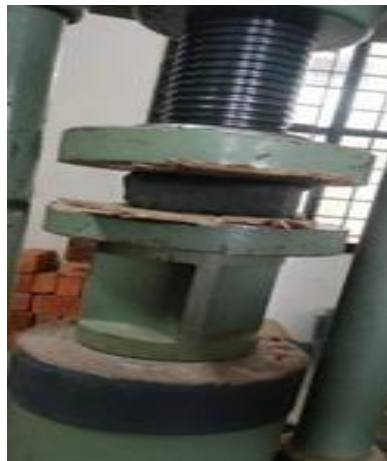
Figure 4: Compressive Strength Testing On Geopolymer Concrete
