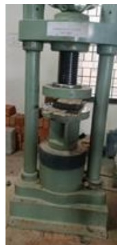
Figure 5: Compressive Strength Testing On Bamboo Reinforced Slab
