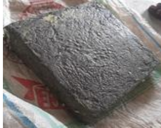
Figure 1: Bamboo Reinforced Geopolymer Concrete Slab
