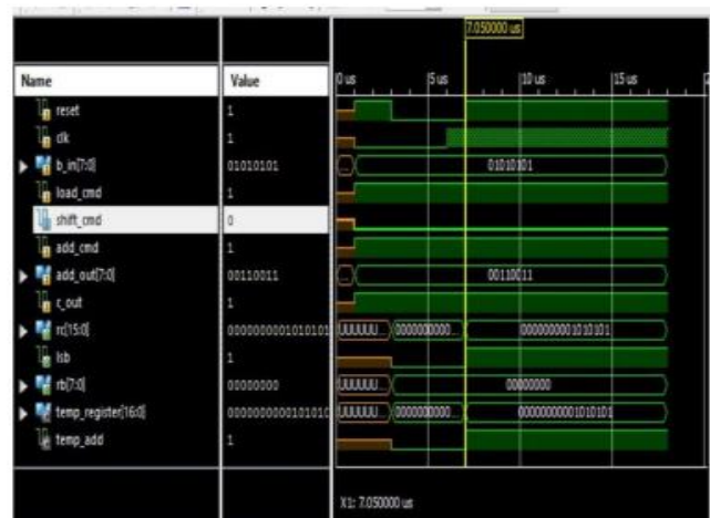
Fig-5: Simulation output in ISim
