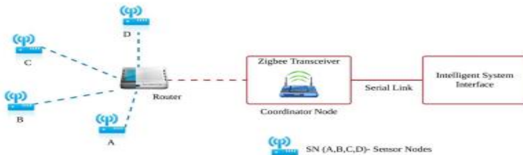
Figure 2: Diagram of Industrial WSN
