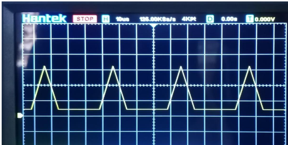
Figure 2: Gate to Source Waveform
