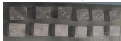
Figure 3: Curing of specimen
