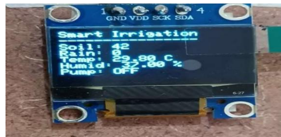
Figure 5: Output of OLED when motor OFF
