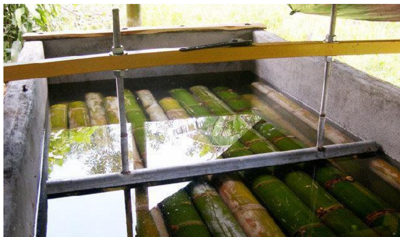
Figure 13: Bamboo immersed in borax boric acid
